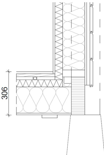
FOR A CONCRETE SLAB FOUNDATION
